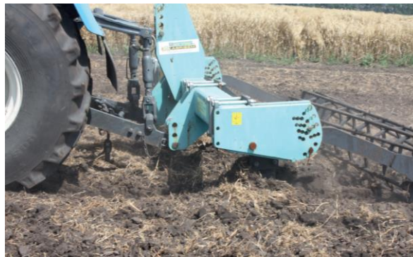
Fig. 2. Appearance of tillage unit with working bodies of parquet type in field experiment
